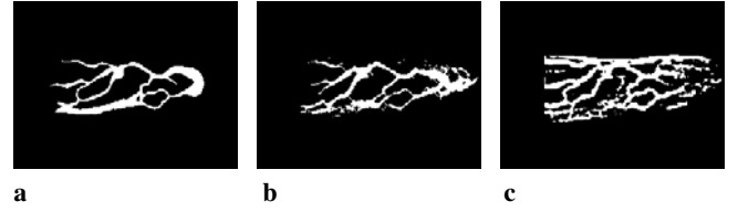
Fig. 9a–c. Finger-vein patterns extracted from Fig. 8a by hand-labeling, and using proposed and conventional methods. a Hand-labeled. b proposed method. c Matched filter
